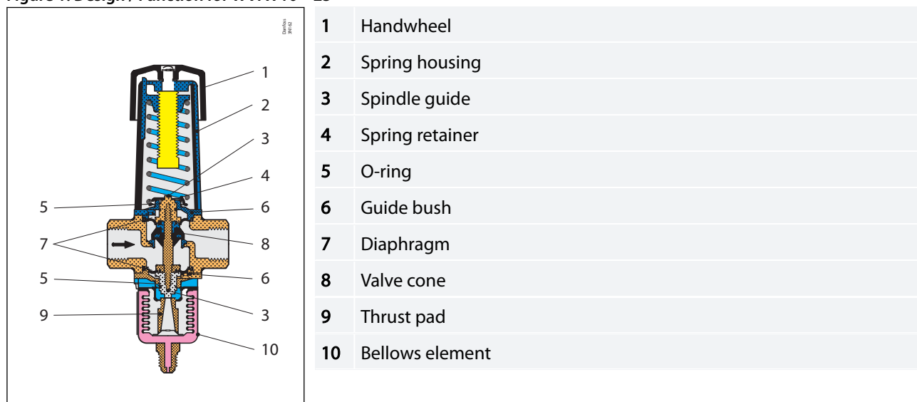
Figure 1: Design / Function for WVFX 10 – 25
